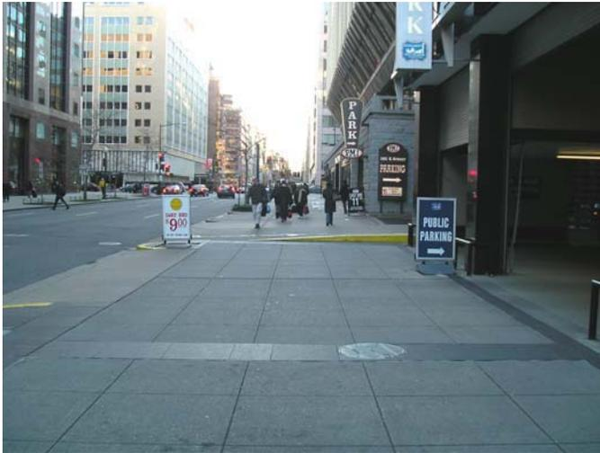
**Figure 3** Colorado Springs, CO – Curb extension with driveway - the design provides a place for drivers to wait for a gap in traffic without blocking pedestrians.
