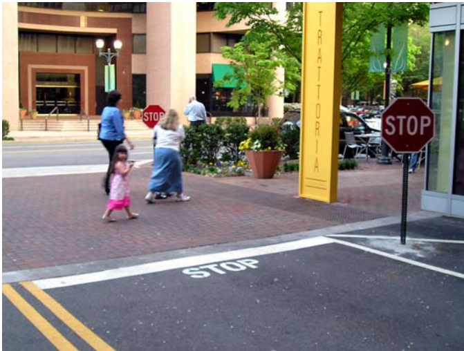
Figure 4 Arlington County, VA – Note the double stop signs, one at the sidewalk and one at the street.
